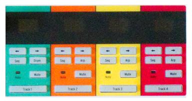
The track controls are identical except for one button: Track 1 has a Drum button for the drum sequencer, but Tracks 2, 3 and 4 each have an Arp button for the arpeggiators. The track controls function as follows:
